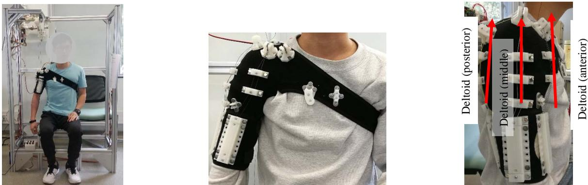
*Fig. 1. Exo-muscular robot prototype. Overall view (left), front view (middle) and side view (right).*
