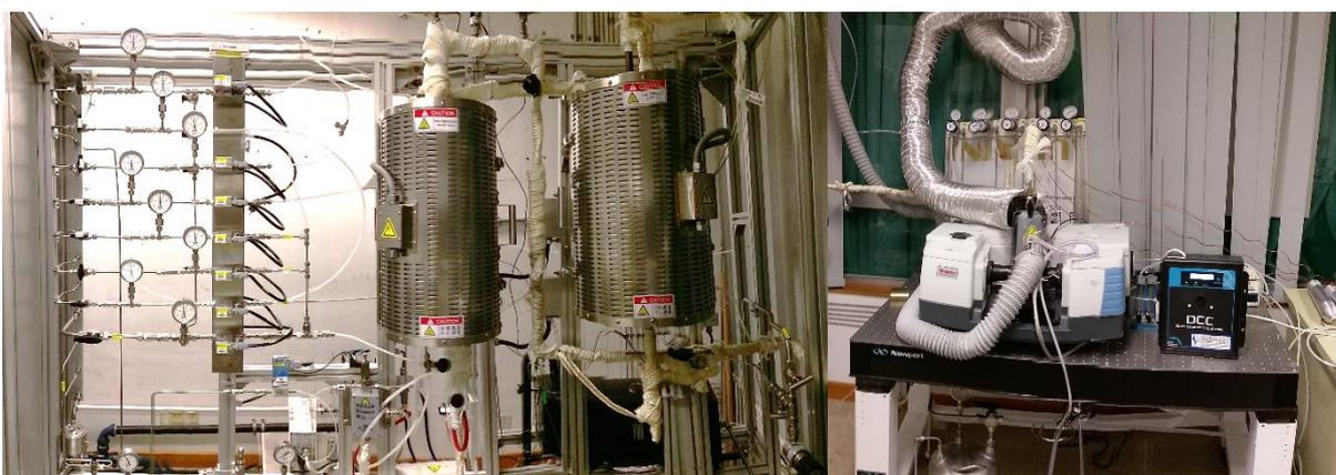
**Figure 1** The catalyst testing system. Left: reactor, gas manifold and steam generator; right: IR spectrometer with 2-m gas cell for gas detection and quantification.
