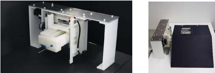
Fig. 3 (left) The fabricated robot prototype. (right) A simulated lateral insertion with a breast coil model
