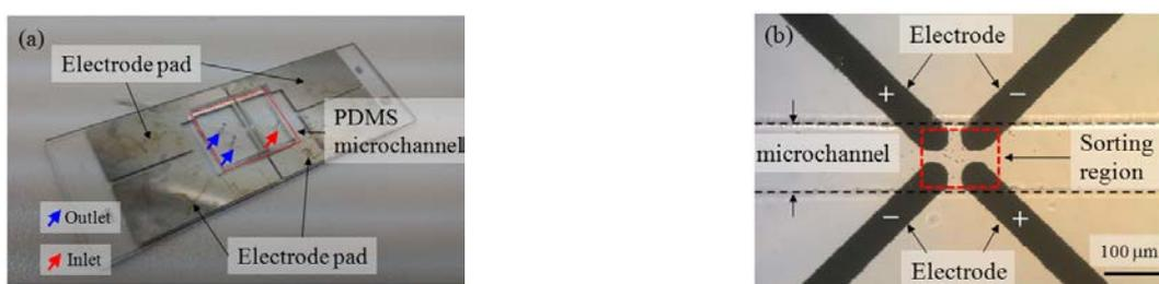
Figure 1: (A) First generation DEP nanoparticle sorting chip; (B) Optical image of electrodes and microchannel.
