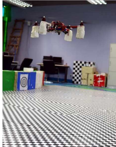
Fig. 3. The UAV autonomously accomplishes hovering and trajectory tracking using onboard sensing.
