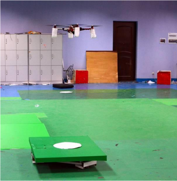
Fig. 2 (d). The UAV autonomously tracks the moving UGV platform via the visual-based approach.
